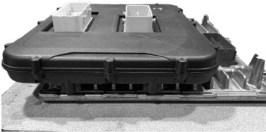
**STEP 3** - Using the 4 supplied aluminum “w” style mounting tabs and 4 small screws, secure the Pulsar to the PCM (see picture)
