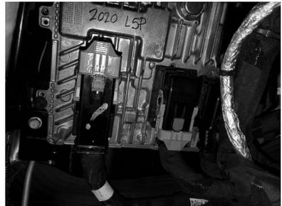
**STEP 5** - Using a 7mm socket, remove the 4 bolts holding the ECM in place (two on the right and two on the left side). Make sure to support the ECM when you remove the bolt as it will drop once the last bolt is removed.
