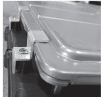
**STEP 4** - Install the Pulsar Mounting Plate to the truck: Remove the lower left 13mm bolt holding the Stock PCM bracket in place. Install the Pulsar Mount Plate between the stock bracket and the frame mount (see picture below) with the 90-degree tab to the top going through the slot in the stock ECM bracket. Reinstall the 13mm bolt while making sure the Pulsar Mounting bracket is level with the stock bracket (see picture below).
